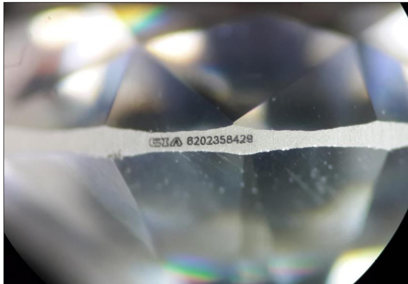
Laser inscription on Synthetic Moissanite
