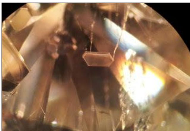
Hexagonal negative cavity in Synthetic Moissanite with extended hollow tube.
