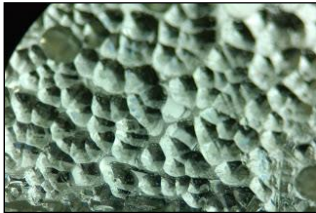
Sub-hexagonal depressions, note irregular sharp pits present between depressions
