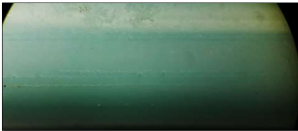
Gas bubbles and swirl marks in glass imitation of Turquoise
