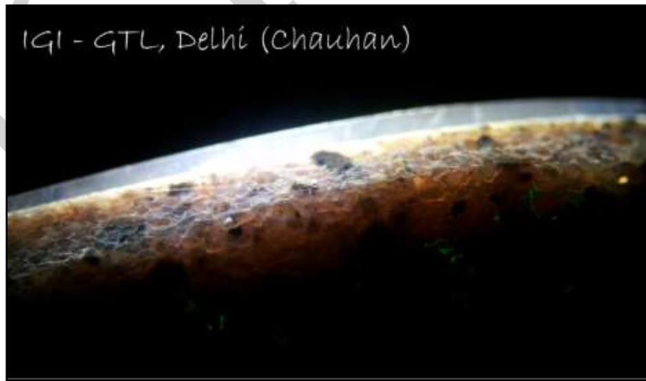
Coat of polymer of approx. thickness 0.5 mm is visible on edge. Under white LED light.
