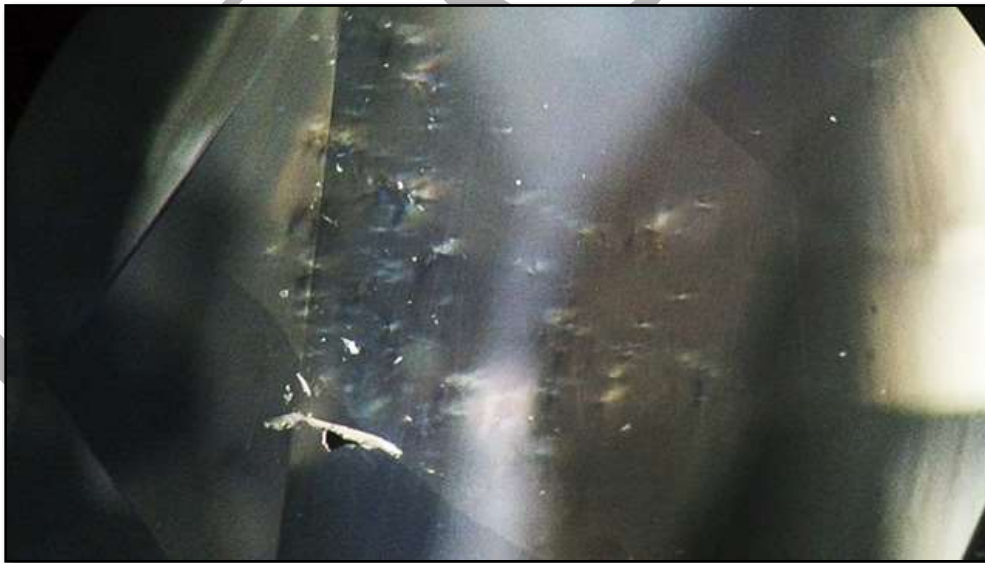
Figure 3. These small stress points, visible on the table between crossed polarizers, were confined to a small space. Photomicrograph by Meenakshi Chauhan; magnified 30 \times .
