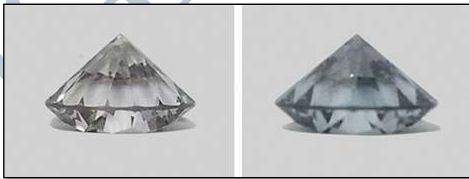
Figure 3. The CVD synthetic diamond before (left) and after exposure (right) to the short-wave UV radiation of the DiamondView. Photos by Meenakshi Chauhan.
