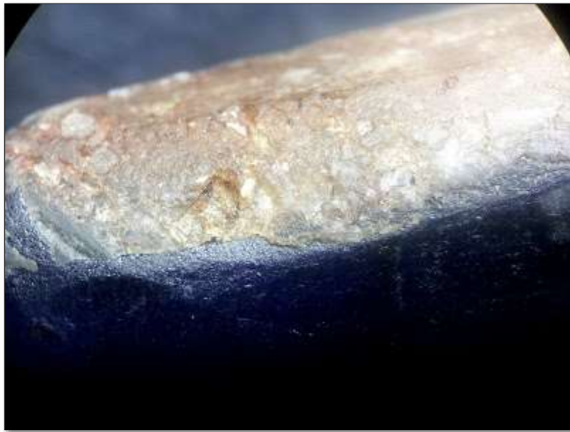
Junction plane of Synthetic Sapphire and fake mother rock, appearing like deliberately pasted material.
