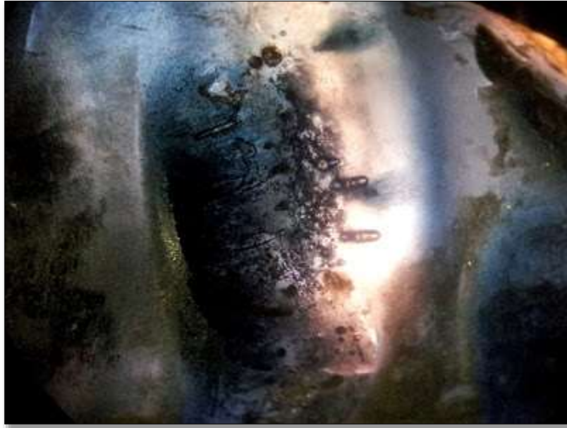
Bunch of round and bullet like Gas Bubbles in Doctored Synthetic Sapphire, evident after applying Pseudo polish.
